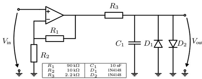
Figure 1: Circuit of the diode clipper with pre-amplification.
