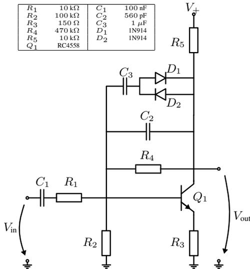
Figure 2: Circuit of a Big Muff transimpedance gain stage.
