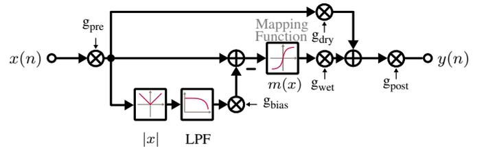
Figure 6: Nonlinear mapping function with extensions.
