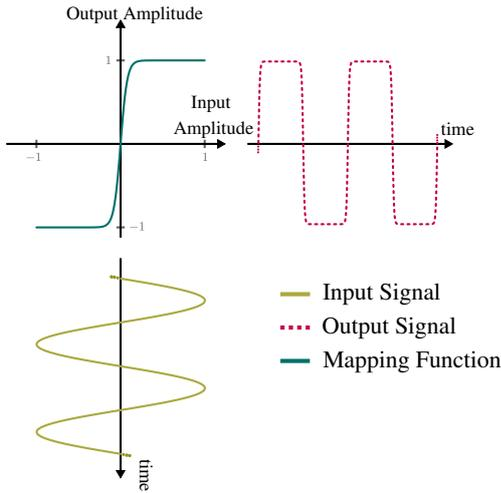
Figure 5: Function principle of a static mapping curve.
